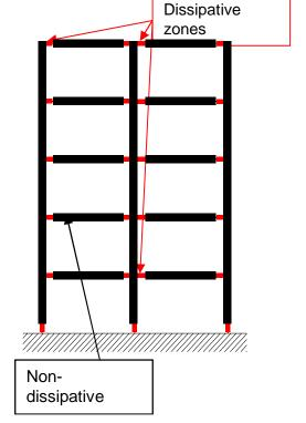
• Detailing of dissipative zones need to supply curvature ductility/local ductility  $\mu_{\phi}$ ; overstrength rules need to be sufficient to concentrate plasticity in dissipative zones only.
